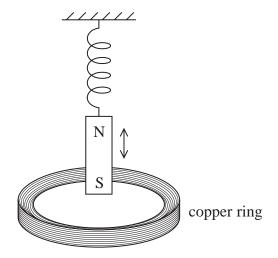
The magnet is displaced vertically and released so that it oscillates. Explain why this produces an alternating current in the copper ring.
