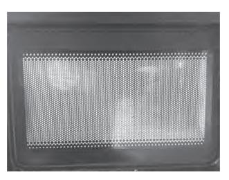
The door consists of two sheets of glass with a layer of metal between. The layer of metal has many small holes in it, so that food inside the microwave oven may be seen while it is being heated without exposing the user to dangerous levels of microwave radiation. It has been suggested that, due to diffraction effects, light can pass through the holes but microwaves cannot.
