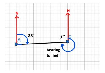
**Step 2**: Using parallel line rules, calculate angle *x*.
