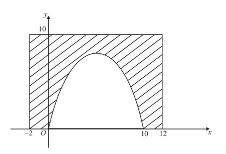
The diagram above shows the cross-section of a road tunnel and its concrete surround. The curved section of the tunnel is modelled by the curve with equation  $y = 8\sqrt{\left(\sin\frac{\pi x}{10}\right)}$ , in the interval  $0 \le x \le 10$ . The concrete surround is represented by the shaded area bounded by the
