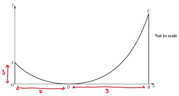
It is required to find the height of pole BC by modelling the shape of the curve that the chain forms.
