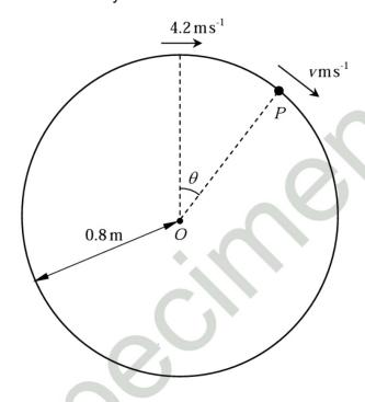
A smooth wire is shaped into a circle of centre O and radius 0.8 m. The wire is fixed in a vertical plane. A small bead P of mass 0.03 kg is threaded on the wire and is projected along the wire from the highest point with a speed of  $4.2\,\mathrm{m\,s}^{-1}$ . When *OP* makes an angle  $\theta$  with the upward vertical the speed of *P* is vm s<sup>-1</sup> (see diagram). Remember:
