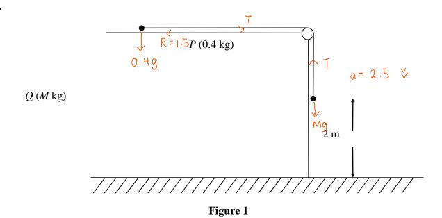
A ball, P, of mass 0.4 kg rests on a rough horizontal table and is attached to one end of a thin rope. The rope passes over a pulley which is fixed at the edge of the table. The other end of the rope is attached to another ball, Q, of mass M kg which hangs freely below the pulley, as shown in Figure 1.
