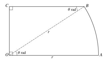
The diagram represents a metal plate OABC, consisting of a sector OAB of a circle with centre O and radius r, together with a triangle OCB which is right-angled at C. Angle  $AOB = \theta$  radians and OC is perpendicular to OA.
