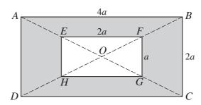
ABCD is a uniform rectangular lamina of mass m in which AB = 4a and BC = 2a. The lines AC and BD intersect at O. The mid-points of OA, OB, OC, OD are E, F, G, H respectively. The rectangle EFGH, in which EF = 2a and FG = a, is removed from ABCD (see diagram). The resulting lamina is free to rotate in a vertical plane about a fixed smooth horizontal axis through A and perpendicular to the plane of ABCD. Show that the moment of inertia of this lamina about the axis is  $\frac{85}{16}ma^2$ . [8]
