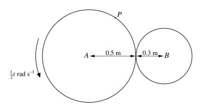
Two coplanar discs, of radii 0.5 m and 0.3 m, rotate about their centres A and B respectively, where AB = 0.8 m. At time t seconds the angular speed of the larger disc is  $\frac{1}{2}t \operatorname{rad} \operatorname{s}^{-1}$  (see diagram). There is no slipping at the point of contact. For the instant when t = 2, find
