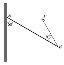
A uniform rod AB of weight W rests in equilibrium with A in contact with a rough vertical wall. The rod is in a vertical plane perpendicular to the wall, and is supported by a force of magnitude P acting at B in this vertical plane. The rod makes an angle of  $60^{\circ}$  with the wall, and the force makes an angle of  $30^{\circ}$  with the rod (see diagram). Find the value of P.
