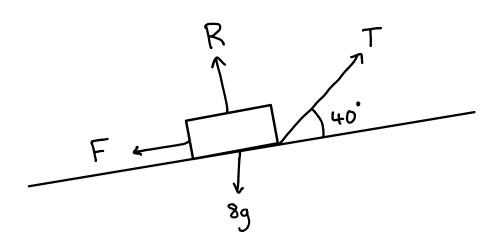
**16 (b) (ii)** Find the tension in the string as the box accelerates up the slope at 3 m s $^{-2}$ .
