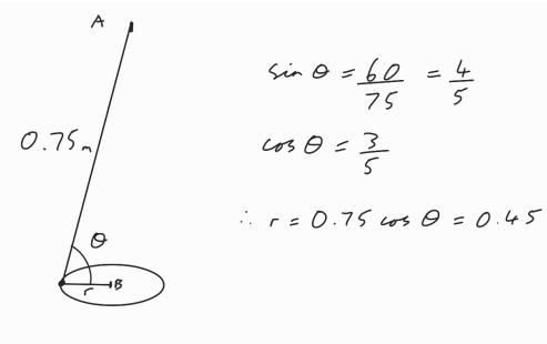
Resolve vertically  $T_1 \sin \theta = 2.5 g$   $T_2 = \frac{25g}{8}$
