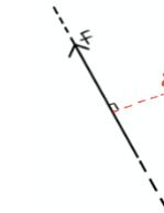
In the above case, the moment is clockwise as the force produces a turning effect in the clockwise direction. Note that since the moment is force (N) multiplied by distance (m), the units for the moment of a force is Nm.
