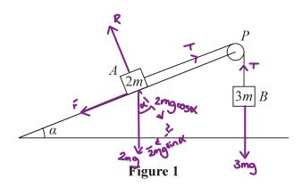
Two blocks, A and B, of masses 2m and 3m respectively, are attached to the ends of a light string.
