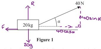
A wooden crate of mass 20 kg is pulled in a straight line along a rough horizontal floor using a handle attached to the crate.
