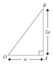
A uniform lamina of mass *M* is in the shape of a right-angled triangle *OAB*. The angle *OAB* is 90°, OA = a and AB = 2a, as shown in the diagram above.
