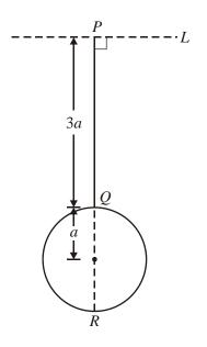
A thin uniform rod PQ has mass m and length 3a. A thin uniform circular disc, of mass m and radius a, is attached to the rod at Q in such a way that the rod and the diameter QR of the disc are in a straight line with PR = 5a. The rod together with the disc form a composite body, as shown in the diagram. The body is free to rotate about a fixed smooth horizontal axis L through P, perpendicular to PQ and in the plane of the disc.
