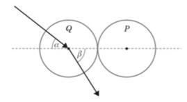
A smooth sphere P lies at rest on a smooth horizontal plane. A second identical sphere Q, moving on the plane, collides with the sphere P. Immediately before the collision the direction of motion of Q makes an angle  $\alpha$  with the line joining the centres of the spheres. Immediately after the collision the direction of motion of Q makes an angle  $\beta$  with the line joining the centres of spheres, as shown in the figure. The coefficient of restitution between the spheres is e.
