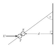
A small smooth uniform sphere S is at rest on a smooth horizontal floor at a distance d from a straight vertical wall. An identical sphere T is projected along the floor with speed U towards S and in a direction which is perpendicular to the wall. At the instant when T strikes S the line joining their centres makes an angle  $\alpha$  with the wall, as shown in the figure.
