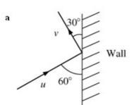
Let the speed of the ball before impact be  $u \text{ m s}^{-1}$  and the speed of the ball after impact be  $v \text{ m s}^{-1}$ .
