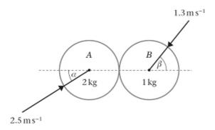
Two smooth uniform spheres A and B of equal radius have masses 2 kg and 1 kg respectively. They are moving on a smooth horizontal plane when they collide. Immediately before the collision the speed of A is  $2.5 \,\mathrm{m \, s^{-1}}$  and the speed of B is  $1.3 \,\mathrm{m \, s^{-1}}$ . When they collide the line joining their centres makes an angle  $\alpha$  with the direction of motion of A and an angle  $\beta$  with the direction of motion of B, where
