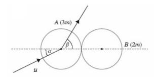
A uniform small smooth sphere of mass 3m moving with speed u on a smooth horizontal table collides with a stationary small sphere B of the same size as A and of mass 2m. The direction of motion of A before impact makes an angle  $\alpha$  with the line of centres of A and B, and the direction of motion of A after the impact makes an angle  $\beta$  with the same line, as shown in the figure. The coefficient of restitution between
