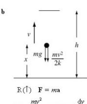
$$-mg - \frac{mv^2}{2k} = ma = mv \frac{dv}{dx}$$
