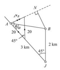
Fix B (apply 20 km h<sup>-1</sup> due N to both) Since velocity  $\Delta$  is isosceles,  $|_{A}\mathbf{v}_{B}| = 40 \sin 22.5^{\circ} = 15.307 \text{ km h}^{-1}$  $\theta = \frac{1}{2} (180^{\circ} - 45^{\circ}) = 67.5^{\circ}$
