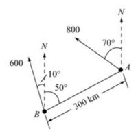
Fix A (i.e. consider motion relative to A) Apply a vector 800 S70°E to both: by cos rule,  $|_{B}\mathbf{v}_{A}|^{2} = 600^{2} + 800^{2} - 2 \times 600 \times 800 \cos 60^{\circ}$ = 520 000
