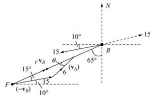
Fix the ball (i.e. consider motion relative to the ball) Using sine rule on vector  $\Delta$
