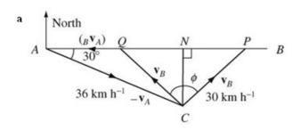
In this diagram, the minimum speed for interception is represented by CN and the maximum speed of A,  $30 \text{ km h}^{-1}$ , by CP and CQ. If  $\angle NCP = \phi$ , then  $\theta$  can vary from  $-\phi$  to  $\phi$ .
