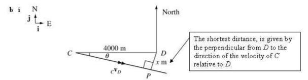
Let the foot of the perpendicular from D to the direction of the velocity of C relative to D be P. Let DP = x m and CP = y m.
