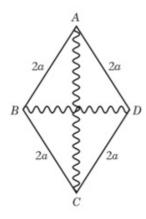
ABCD is a rhombus consisting of four freely jointed uniform rods, each of mass m and length 2a. The rhombus is freely suspended from A and is prevented from collapsing by two light springs, each of natural length a and modulus of elasticity 2mg. One spring joins A and C and the other joins B and D, as shown in the diagram.
