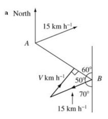
You fix A by introducing a vector equal and opposite to the velocity of A to the system.
