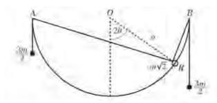
A smooth wire with ends A and B is in the shape of a semi-circle of radius a. The mid-point of AB is O. The wire is fixed in a vertical plane and hangs below AB which is horizontal. A small ring R, of mass  $m\sqrt{2}$ , is threaded on the wire and is attached to two light inextensible strings. The other end of each string is attached to a particle of mass  $\frac{3m}{2}$ . The particles hang vertically under gravity, as shown in the diagram
