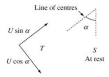
Let the components of velocities after the collision be
