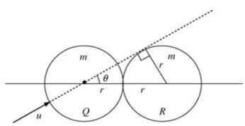
Let the mass of each of the spheres be m and the radius of each of the spheres be r. Let the angle the direction of motion of Q makes with the line of centres before the impact be  $\theta$ .
