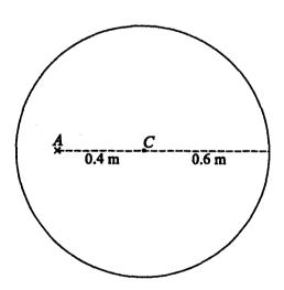
A uniform circular disc has mass 4 kg, radius 0.6 m and centre C. The disc can rotate in a vertical plane about a fixed horizontal axis which is perpendicular to the disc and which passes through the point A on the disc, where AC = 0.4 m. A frictional couple of constant moment 4.8 N m opposes the motion. The disc is released from rest with AC horizontal (see diagram).
