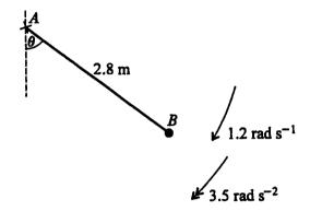
At one instant, AB makes an acute angle  $\theta$  with the downward vertical, the angular speed of the body is 1.2 rad s<sup>-1</sup> and the angular acceleration of the body is 3.5 rad s<sup>-2</sup> (see diagram).
