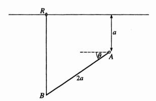
The diagram shows a uniform rod AB, of mass m and length 2a, free to rotate in a vertical plane about a fixed horizontal axis through A. A light elastic string has natural length a and modulus of elasticity  $\frac{1}{2}mg$ . The string joins B to a light ring R which slides along a smooth horizontal wire fixed at a height a above A and in the same vertical plane as AB. The string BR remains vertical. The angle between AB and the horizontal is denoted by  $\theta$ , where  $0 < \theta < \pi$ .
