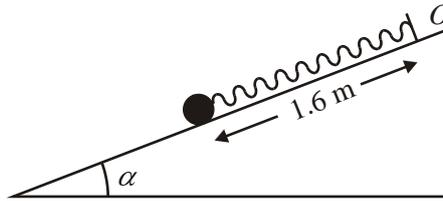
A particle of mass 0.8 kg is attached to one end of a light elastic spring, of natural length 2 m and modulus of elasticity 20 N. The other end of the spring is attached to a fixed point  $O$  on a smooth plane which is inclined at an angle  $\alpha$  to the horizontal, where  $\tan \alpha = \frac{3}{4}$ . The particle is held on the plane at a point which is 1.6 m down a line of greatest slope of the plane from  $O$ , as shown in the diagram. The particle is then released from rest.
