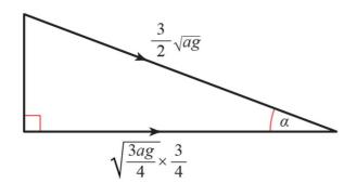
After leaving the hemisphere the horizontal component of the velocity remains constant.
