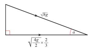
After leaving the hemisphere the horizontal component of the velocity remains constant. Direction is angle  $\alpha$  to the ground,
