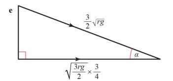
After leaving the hemisphere the horizontal component of the velocity remains constant.
