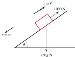
Resolving parallel to the slope and using F = ma: 1000-750×9.8×sin $\theta$  = 750*a*
