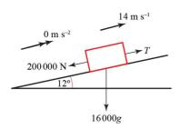
Resolving parallel to the slope:  $T = 200000 + 16000g \sin 12^{\circ}$   $T = 232600.5\cdots$ Work done in 10 s = force x distance moved
