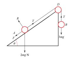
a P.E. gained by A = mgh  $= 2mg \times (s \times \sin \theta)$   $= 2mg \times s \times \frac{3}{5}$   $= \frac{6mgs}{5}$ P.E. lost by B = mgh = 3mgs $\therefore$  P.E. lost by system  $= 3mgs - \frac{6mgs}{5} = \frac{9mgs}{5}$
