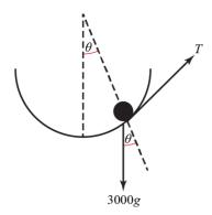
**a** Car is moving with constant speed in a direction along the tangent to the cylinder. Resolving along the path of the car:
