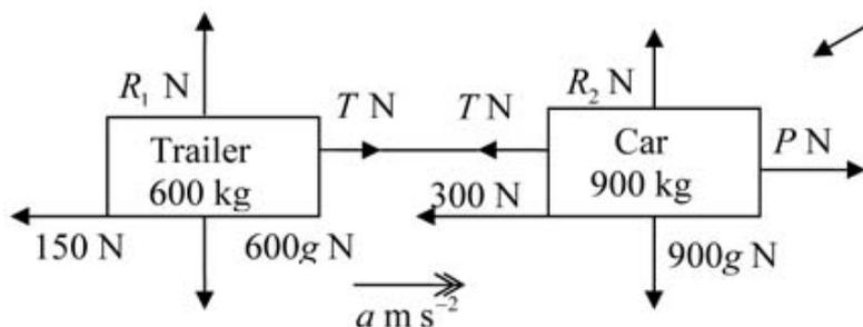
The tractive force exerted by the engine of the car has been called  $P$  N. This only acts on the car. It does not act directly on the trailer. The only force moving the trailer forward is the tension in the tow bar.
