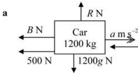
The force exerted by the brakes is labelled as  $B$  N in this diagram. During braking both the braking force and the resistance act to slow the car down.
