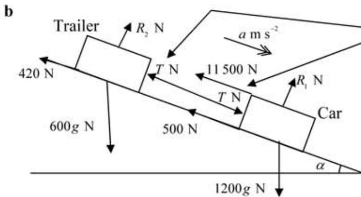
Under braking, the force in the tow bar is a thrust and acts outwards in the directions shown in the diagram. When Newton's second law is applied to the whole system, the forces at the ends of the tow bar are of equal magnitude and in opposite directions and so they cancel one another out.
