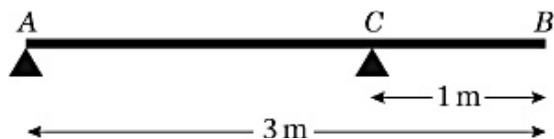
A uniform beam  $AB$  has mass 12 kg and length 3 m. The beam rests in equilibrium in a horizontal position, resting on two smooth supports. One support is at end  $A$ , the other at a point  $C$  on the beam, where  $BC = 1$  m, as shown in the diagram. The beam is modelled as a uniform rod.
