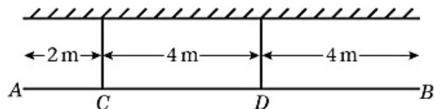
A light rod  $AB$  has length 10 m. It is suspended by two light vertical cables attached to the rod at the points  $C$  and  $D$ , where  $AC = 2$  m,  $CD = 4$  m, and  $DB = 4$  m, as shown in the diagram. A load of weight 60 N is attached to the rod at  $A$  and a load of weight  $X$  N is attached to the rod at  $B$ . The rod is hanging in equilibrium in a horizontal position. Find, in terms of  $X$ ,
