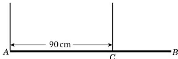
A steel girder  $AB$  has weight  $210\text{ N}$ . It is held in equilibrium in a horizontal position by two vertical cables. One cable is attached to the end  $A$ . The other cable is attached to the point  $C$  on the girder, where  $AC = 90\text{ cm}$ , as shown. The girder is modelled as a uniform rod, and the cables as light inextensible strings.
