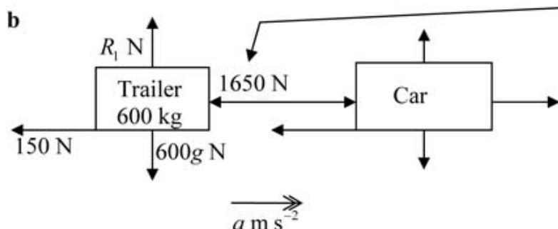
When decelerating the force in the tow bar becomes a thrust. The question gives that the greatest magnitude of the thrust is 1650 N. To solve part b, you need only the horizontal forces on the trailer.
