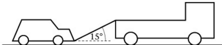
The figure above shows a lorry of mass 1600 kg towing a car of mass 900 kg along a straight horizontal road. The two vehicles are joined by a light tow-bar which is at an angle of  $15^\circ$  to the road. The lorry and the car experience constant resistances to motion of magnitude 600 N and 300 N respectively. The lorry's engine produces a constant horizontal force on the lorry of magnitude 1500 N. Find
