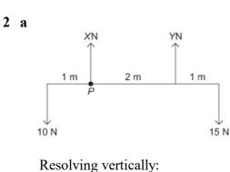
X + Y = 10 + 15= 25 Taking moments about P:  $15 \times (2+1) = 10 \times 1 + Y \times 2$ 45 = 10 + 2Y2Y = 35Y = 17.5 $\Rightarrow X = 7.5 \text{ and } Y = 17.5$
