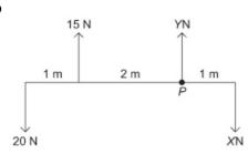
Resolving vertically: 15+Y=20+X Y-X=5Taking moments about P:  $20 \times (2+1) = 15 \times 2 + X \times 1$  60 = 30 + X X = 30 $\Rightarrow X = 30$  and Y = 35
