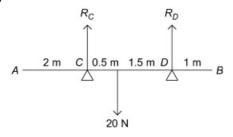
Resolving vertically:  $R_C + R_D = 20$ Taking moments about C :  $R_D \times 2 = 20 \times 0.5$  = 10 $\Rightarrow R_D = 5 \text{ N}$  and  $R_C = 15 \text{ N}$
