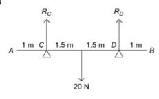
Resolving vertically:  $R_C + R_D = 20$ Taking moments about C :  $3 \times R_D = 1.5 \times 20$  = 30 $\Rightarrow R_D = 10$  N and  $R_C = 10$  N
