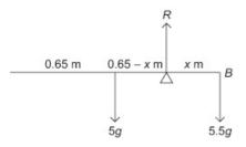
Let the support be x m from the broomhead. Taking moments about the support:  $5.5g \times x = 5g \times (0.65 - x)$  $5.5x = 5 \times 0.65 - 5x$ 10.5x = 3.25x = 0.31
