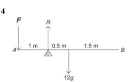
Suppose that the force required is *F* N acting vertically downwards at *A*. Taking moments about the pivot (*C*):  $F \times 1 = 0.5 \times 12g$
