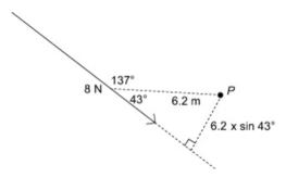
First, draw in the right-angled triangle. Angle inside the triangle =  $180^{\circ} - 137^{\circ} = 43^{\circ}$
