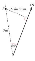
First, draw in the right-angled triangle. Perpendicular distance =  $5 \times \sin 30^{\circ}$ Moment =  $4 \times 5 \sin 30^{\circ}$
