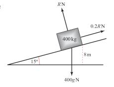
To show that the boat will slide back down the slipway, we need to show that the component of weight acting down the slope is greater than the limiting friction:
