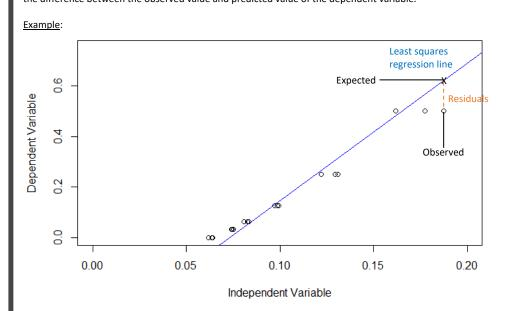
The least squares linear regression can be used to estimate the corresponding value of the dependent variable for a value of the independent variable. It can be written in the form:
