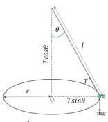
The motion of a conical pendulum is an example of three-dimensional horizontal circular motion. It consists of simple pendulum with a string or rod of length *l* attached to a fixed pivot with a bob/weight of mass m at the other end of the string or rod. The bob can be imagined as moving round in a circle at a constant angular speed  $\omega$  while the string or rod traces out the cone shape creating an angle  $\theta$  between the string and the vertical component.
