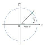
A particle moving in a horizontal circular orbit can have its displacement, velocity and acceleration described by vectors. Consider a particle moving in a horizontal circular path in the xy-plane, as seen in the diagram on the left. The position of the particle has both x and y coordinates, so is written as the position vector in terms of the angle  $\varphi$ measured anticlockwise from OA or the constant angular speed  $\omega$  and time. t:
