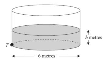
The diagram above shows a cylindrical water tank. The diameter of a circular cross-section of the tank is 6 m. Water is flowing into the tank at a constant rate of  $0.48\pi$  m<sup>3</sup> min<sup>-1</sup>. At time t minutes, the depth of the water in the tank is h metres. There is a tap at a point T at the bottom of the tank. When the tap is open, water leaves the tank at a rate of  $0.6\pi$  h m<sup>3</sup> min<sup>-1</sup>.
