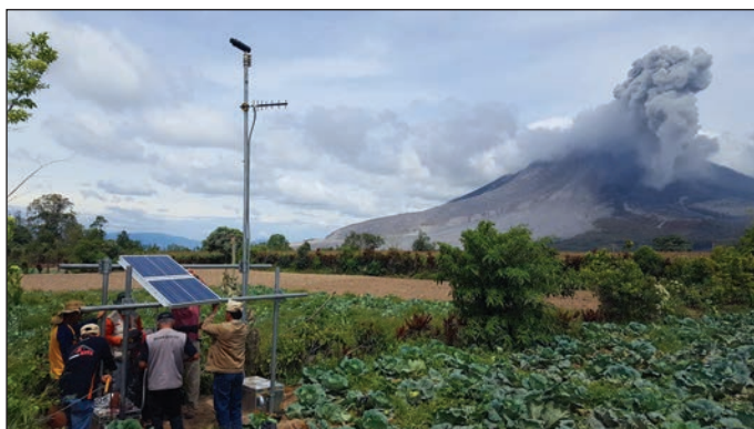
Figure 6d: Installing volcano monitoring equipment in Indonesia
