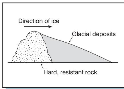
Figure 5: Cross-section of a crag and tail
