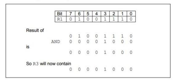
Figure 3 – Example when bit 3 of R1 contains a 0
