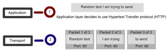
The transport layer separates the packets, and labels them appropriately it also includes the port number so that the recipients computer can handle the data appropriately
