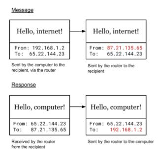
NAT gets around this problem. When a device on the private network (let's use 192.168.1.2) needs to communicate with a device on the Internet (let's use the server), it sends packets through the router, which makes a record of the packet before replacing the private IP address of the computer with its own routable IP address.
