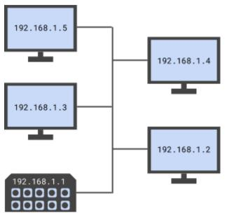
Networks can be divided into smaller networks, called subnets. Each subnet has a different network identifier.
