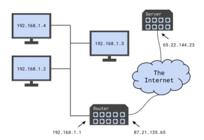
If a device on the network sent a packet to the server, the server couldn't respond to the computer directly because the computer's IP address is non-routable - not globally unique.
