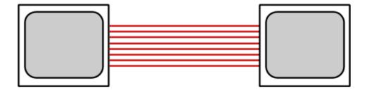
The more lines that a parallel communication medium uses, the more data can be transferred simultaneously.
