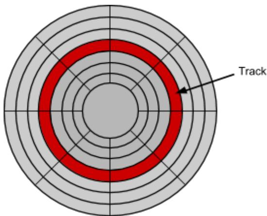
Data is written in **concentric tracks**, each of which is further divided into **sectors**. The platter rotates **thousands of times per minute**, allowing for good read and write speeds.
