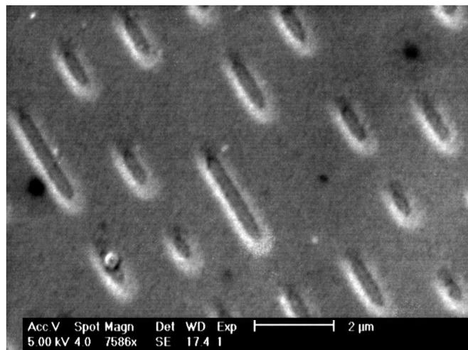
Unlike hard-disk drives which use tracks and sectors, optical disks have **just one continuous track** which **spirals** from the center of the disk to the outside edge.
