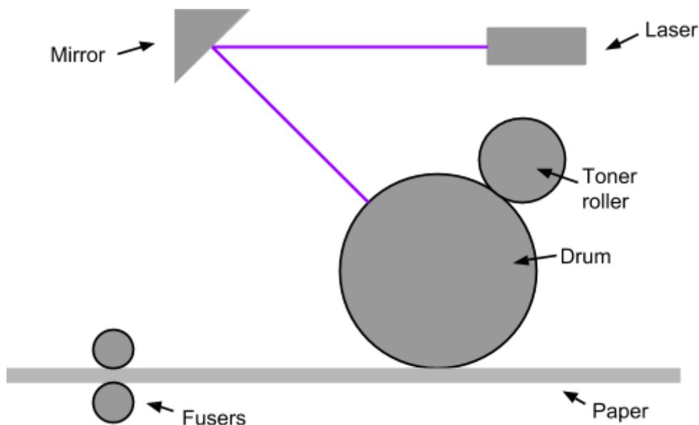
When a document is printed, the drum is [electrically charged](#) all over before the laser is directed at its surface by the mirror. Areas on which the laser is incident are [discharged](#), leaving behind an [impression of the page](#) in electrical charge on the drum.
