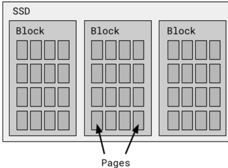
Unlike hard disk drives, SSDs are **not capable of overwriting** data. Instead, an SSD's controller must **completely erase** the entirety of a page before writing **new information** to it.
