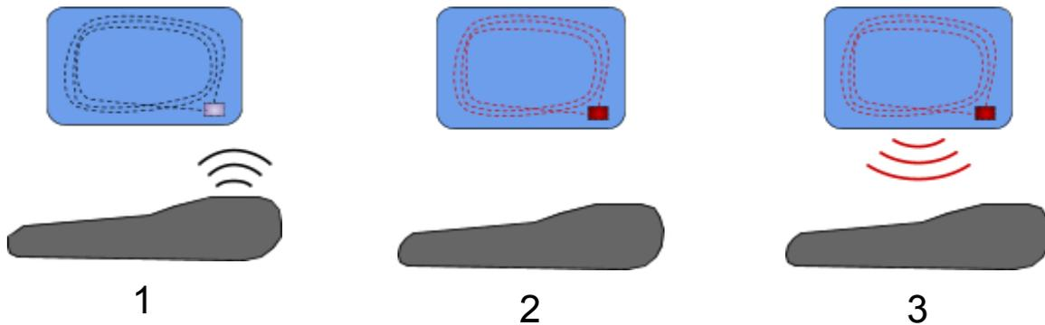
When an RFID tag is scanned, the reader emits **radio waves** which are picked up by the tag's antenna (stage 1). The power induced in the tag's antenna from these waves is enough to power the chip (stage 2) which then uses its antenna to emit its own radio wave (stage 3), which contains the information held on the chip. This wave is picked up by the reader which **decodes** the information and returns the information to a computer.
