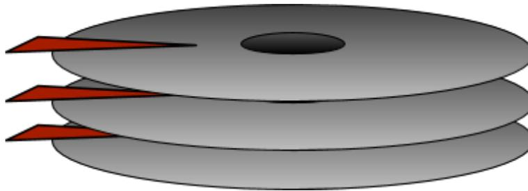
The actuating arm allows the read/write head, which changes the magnetic **polarity** of parts of the platter, to access **all portions** of each platter.
