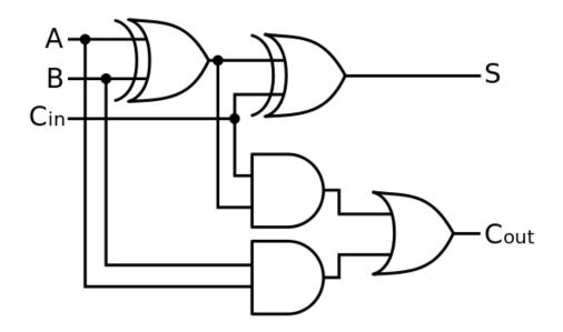
The three inputs are labelled A, B and  $C_{in}$  for carry in. The two outputs are labelled S for sum and  $C_{out}$  for carry out.
