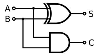
The two inputs are labelled A and B and the outputs are labelled S and C. Short for sum and carry.
