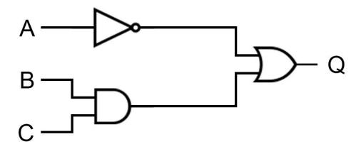
The logic circuit above combines three logic gates and can be represented using the logical expression below.
