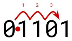
Next, treating the number as if there were a binary point between the first and second digits of the mantissa, move the binary point the number of positions specified by the exponent. In this case, the binary point moves three positions.
