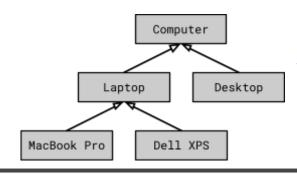
Inheritance is shown with unfilled arrows which point from an inherited class towards the class which inherits it. In this example, the Laptop class inherits the Computer class so an arrow points upwards from Laptop to Computer.
