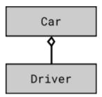
Aggregation (the weaker of the two types of association) is shown with an unfilled diamond headed arrow.
