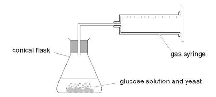
The experiment was carried out three times at five different temperatures. The volume of gas collected after 10 minutes was recorded each time. The results are shown below.
