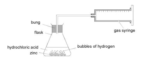
A few pieces of zinc were placed in excess dilute hydrochloric acid and the volume of hydrogen produced was recorded every 10 seconds. The experiment was carried out at room temperature. The results obtained are shown below.
