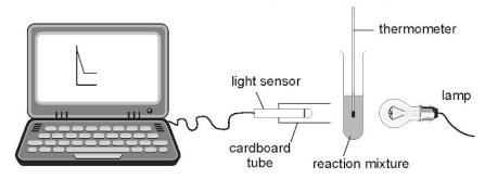
5 cm³ of dilute hydrochloric acid was added separately to 10 cm³ sodium thiosulfate solutions at four different temperatures. All other factors were kept the same. The results are shown on the grid below.
