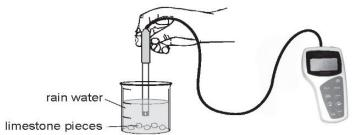
They added limestone pieces to the rain water and recorded the pH of the mixture for 5 minutes. The data collected was then downloaded to a computer.
