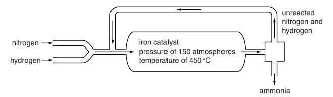
(a) Unreacted nitrogen and hydrogen are recycled.
