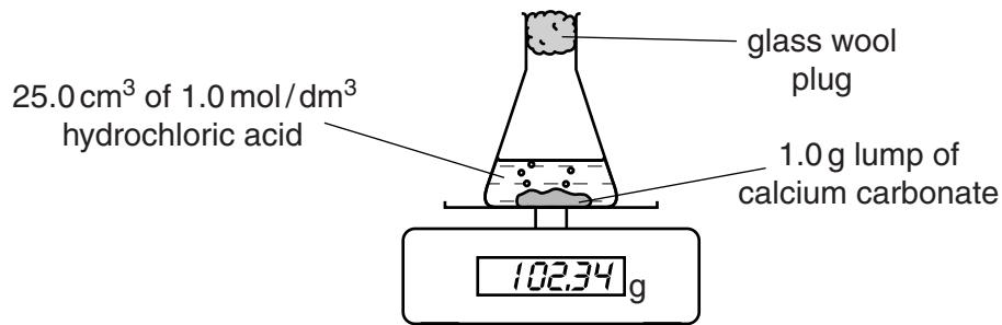
This apparatus can be used to find the mass of carbon dioxide made during the reaction.
