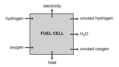
(a) In this fuel cell, hydrogen,  $H_2$ , reacts with oxygen,  $O_2$ .
