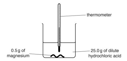
The temperature of the acid before the magnesium is added is 22.0 °C.
