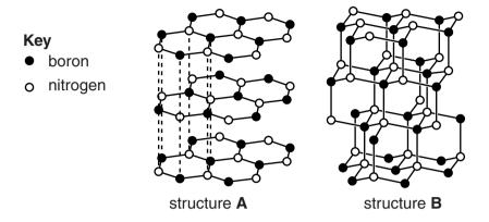
These two forms of boron nitride resemble graphite and diamond, the two allotropes of carbon.
