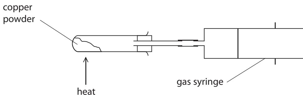
The copper powder in the test tube was heated strongly so that it could react with oxygen in the air in the apparatus.
