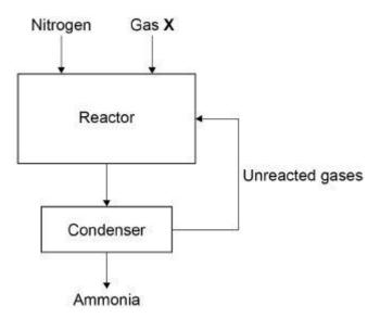
(a) Gas **X** in the diagram above is obtained from methane.
