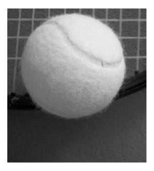
'Nanocoated' tennis balls have a 'nanosize' layer of butyl rubber. This layer slows down the escape of air so that the ball does not lose its pressure as quickly. The 'nanocoated' tennis balls last much longer and do not need to be replaced as often.
