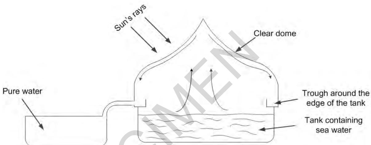
The diagram shows a cross-section through a solar still.
